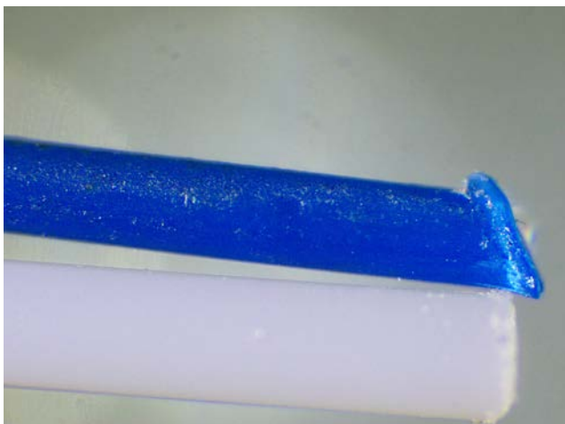
Cimex Nylon Carpet Bristle (.50mm Denier) Compared to CRB Polypropylene Bristle (.35mm Denier) - The CRB brush is only recommended for yearly or restorative cleaning.
